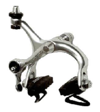
Rim brakes, power brakes or V brakes are calliper brakes that work by pinching the bicycle rim between two blocks of brake pads.
